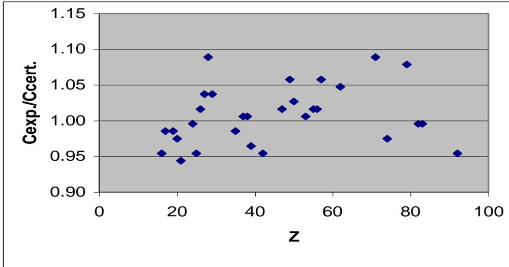
**Figure 4. A fixed H value for PIXE measurements is determined from the ratio of the experimental concentration over the certified one, as function of the atomic number from S to U using Micromatter thin film standards.**
