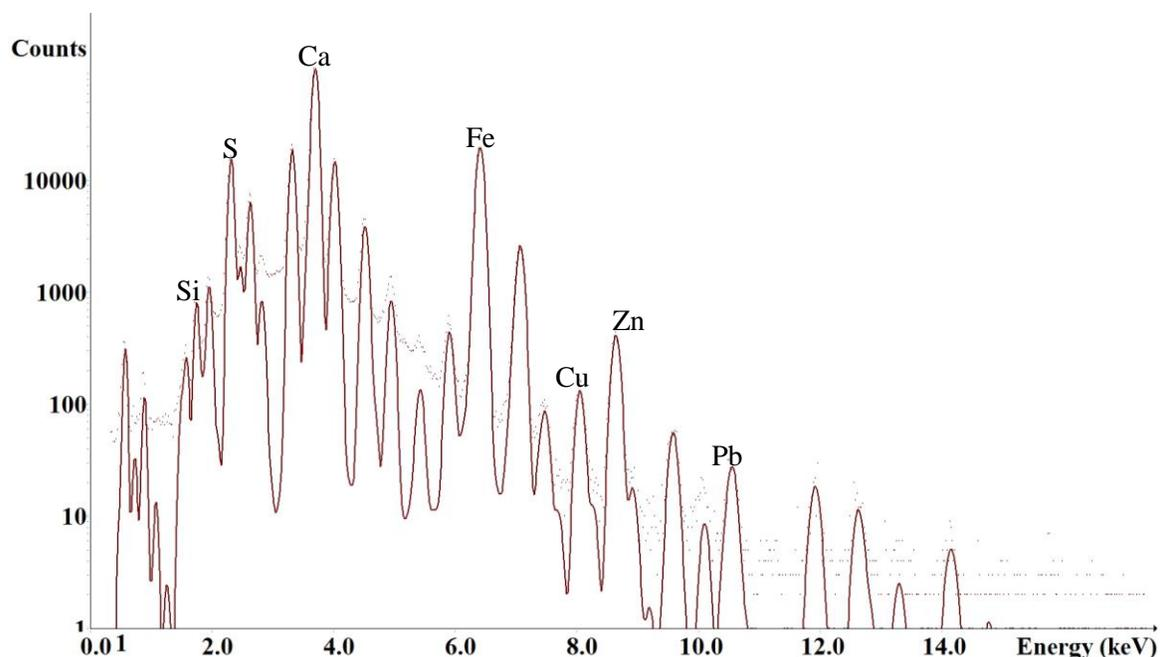
**Figure 5. Typical PIXE spectrum of PM2.5-Teflon filter using Amptek SDD. It represents the acquired experimental spectrum with the fitted one using Gupixwin code**
