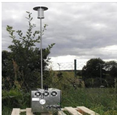
**Figure 2. Microprocessor Controlled Aerosol Sampling device ISAP 1050e with combined inlet for PM<sub>10-2.5</sub> and PM<sub>2.5</sub>**
